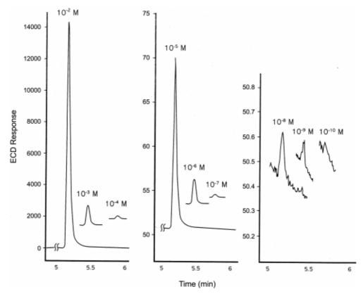
Figure 1. Chromatograms of the standard solutions of the secondary derivatives. The GC operating conditions: splitless injection using an autoinjector (1 μL), 250 °C; carrier gas, helium; oven temperature, from 120 °C to 200 °C at 20 °C/min; detector (ECD) temperature, 320 °C.
