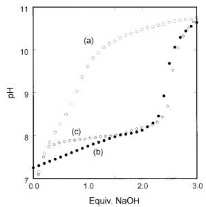
Figure 1. Potentiometric titration curves (c = 0.40 mM): (a) [1Eu]Cl<sub>3</sub>. (b) [2Eu]Cl<sub>3</sub>. (c) EuCl<sub>3</sub>  $\cdot$  6H<sub>2</sub>O.
