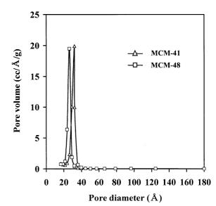
**Figure 2.** Pore size distribution curves of calcined MCM-41 and calcined MCM-48 calculated from the desorption branch of the nitrogen adsorption isothem using the BJH formula.
