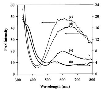
Figure 9. Photoacoustic spectra of (a) Ni/APTMS/MCM-41, (b) Ni/AAPTMS/MCM-41, (c) Cu/APTMS/MCM-41, and (d) Cu/AAPTMS/MCM-41.
