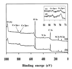
**Figure 8.** X-ray photoelectron spectra of (a) Co/APTMS/MCM-41 and (b) Co/AAPTMS/MCM-41. Inset shows the smoothed and enlarged XP spectra of the cobalt 2p photoelectron region of (c) spectrum (a) and (d) spectrum (b).
