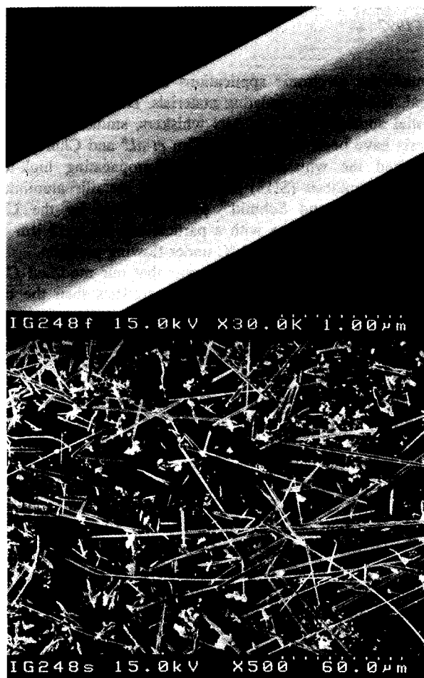
Figure 2. Scanning electron micrographs of AlN whiskers obtained by calcination of (hydroxo)succinato)Al(III) at 1500 °C for 20 h in an N_2 atmosphere.
