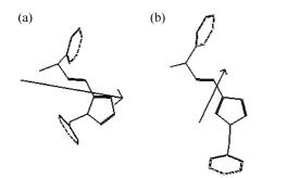
**Figure 1.** The direction and size of dipole moment of (a) 1-benzyltetrazolylimine (size: 4.64 debye) and (b) 2-benzyltetrazolylimine (size: 2.19 debye).
