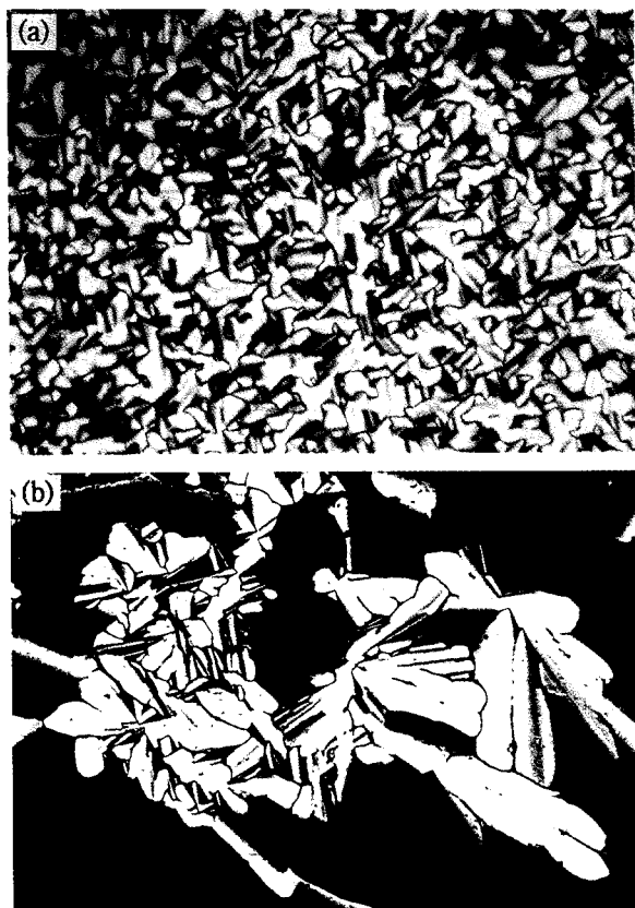
Figure 3. Representative optical polarized micrographs (100X) of the texture exhibited by the columnar mesophase of (a) 6 at 67 °C on the cooling scan and (b) 10 at 74 °C on the cooling scan.
