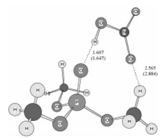
**Figure 1.** Structure of TMP-HNO<sub>3</sub> optimized at the MP2 and HF level using 6-31G(d,p) basis sets. Bond lengths are in Å. Numbers in parenthesis are obtained from the HF level.
