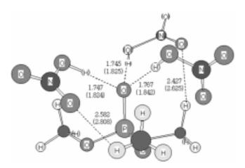
**Figure 3.** Structure of TMP-(HNO<sub>3</sub>)<sub>3</sub> optimized at the MP2 and HF levels using 6-31G(d,p) basis sets. Bond lengths are in Å. Numbers in parenthesis are obtained from the HF level.
