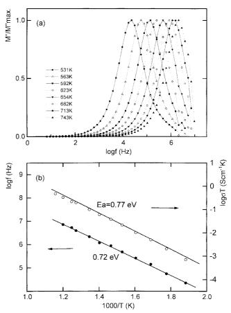
**Figure 4.** Normalized M'' vs.  $\log f$  (Hz) of  $Na_{0.80}Co_{0.40}Ti_{1.60}O_4$  at various temperatures (a) and plots of  $\log T$  and  $\log f_{\max}$  (Hz) vs. 1000/T(K) (b).
