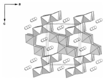
**Figure 1**. Structure of  $Na_xFe_xTi_{2-x}O_4$  (0.72  $\leq x \leq 0.90$ ).  $Fe^{3+}$  and  $Ti^{4+}$  ions are considered as statistically distributed in octahedral sites and  $Na^+$  ions (balls) are partially present in the tunnel along **b**-axis.
