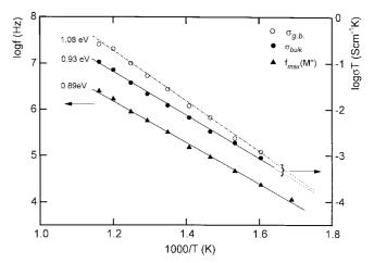
**Figure 6.** Normalized M'' vs.  $\log f(\mathrm{Hz})$  of  $\mathrm{Na}_{0.80}\mathrm{Ni}_{0.40}\mathrm{Ti}_{1.60}\mathrm{O_4}$  at various temperatures (a) and plots of  $\log T$  and  $\log f_{\mathrm{max}}(\mathrm{Hz})$  vs.  $1000/\mathrm{T(K)}$ .
