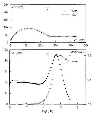
**Figure 5.** Cole-Cole diagram of  $Na_{0.80}Ni_{0.40}Ti_{1.60}O_4$  at 800 K with the fitting-curve (a) and combined Z'' and normalized M'' plots as a function of frequency (b).
