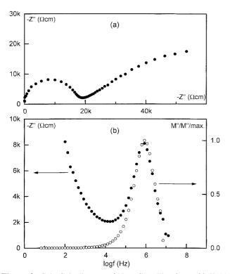
**Figure 3**. Cole-Cole diagram of  $Na_{0.80}Co_{0.40}Ti_{1.60}O_4$  at 682 K (a) and combined Z'' and normalized M''' plots as a function of frequency (b).
