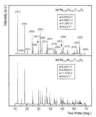
**Figure 2.** Powder X-ray diffraction patterns of Na<sub>0.80</sub>M<sub>0.40</sub>Ti<sub>1.60</sub>O<sub>4</sub> (M=Co or Ni). Some selected peaks are labeled with Miller index.
