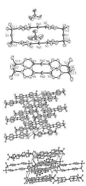
**Figure 1**. ORTEP view of plate [AgL]<sub>2</sub>(ClO<sub>4</sub>)<sub>2</sub>, indicating two inequivalent molecules in the unit cell (top). Packing diagram of needle (middle) and plate crystals (bottom). For each structure, hydrogen atoms are omitted for clarity.
