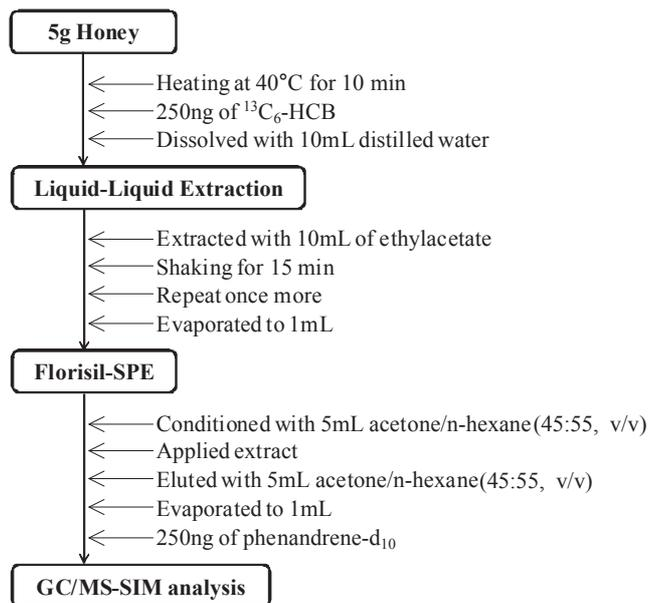
**Figure 2.** Analytical procedures for the determination of acaricides in honey samples.
