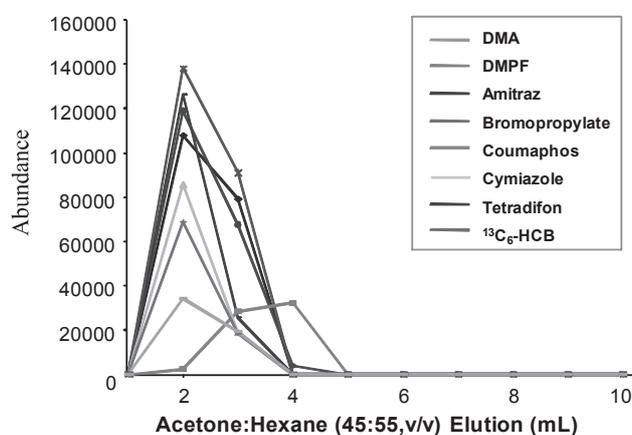
Figure 5. Elution patterns of acaricides and amitraz-degradation products on the Florisil cartridge with the elution of acetone/*n*-hexane mixture (v/v, 45:55)
