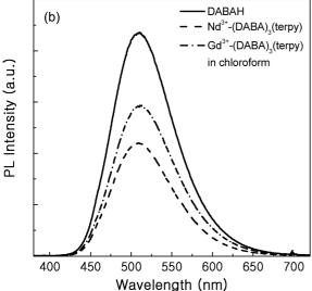
**Figure 3**. Emission spectra of DABAH and Ln<sup>3+</sup>-(DABA)<sub>3</sub>(terpy) (concentration =  $2 \times 10^{-5}$  M) with an excitation at 350 nm.
