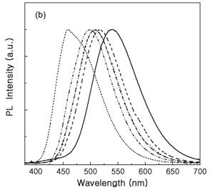
**Figure 1**. Absorption (a) and emission (b) spectra of DABAH in various solvents (concentration =  $2.0 \times 10^{-5}$  M) with an excitation at 350 nm.
