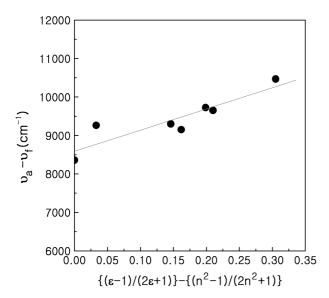
**Figure 2**. The Stokes' shift of DABAH fluorescence as a function of solvent polarity parameters. The number refer to the following solvents: 1; ACN, 2; THF, 3; EA, 4; ethyl ether, 5; chloroform, 6; dioxane, 7; cyclohexane.
