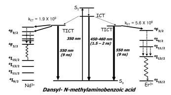
**Scheme 2.** Schematic diagram of the photophysical processes leading to sensitized Ln<sup>3+</sup> luminescence of Ln<sup>3+</sup>-(DABA)<sub>3</sub>(terpy).
