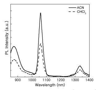
**Figure 4**. Emission spectra of sensitized Nd<sup>3+</sup> ion in Nd<sup>3+</sup>-(DABA)<sub>3</sub>(terpy) with an excitation at 350 nm.
