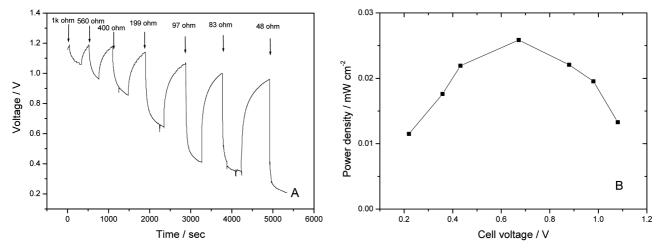
**Figure 6**. Voltage output as a function of different external loads for the two single cells stacked in series. Oxygen reduction reaction was utilized at a cathode. Anodic volume is 150 mL. Each anodic compartment contains 6 mL of *P. vulgaris* suspended solution, 24 mL of 1 mM thionin, 6 mL of 1 mM glucose, and 114 mL of buffer solution.
