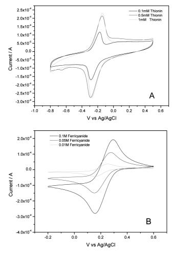
**Figure 3**. Cyclic voltammograms of thionin (panel A) and  $Fe(CN)_6^{3-}$  (panel B) in pH 7 phosphate buffer at a carbon electrode. Both show the reversible redox behaviors.
