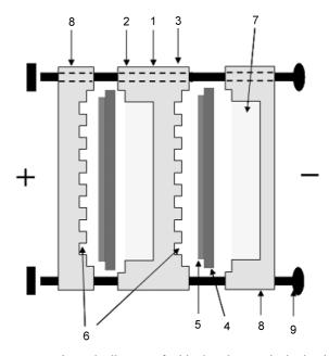
**Figure 2**. Schematic diagram of a bipolar plate stacked microbial fuel cell. Two single cells are connected in series. Anodic compartment (170 mL) contains *P. vulgaris*, glucose and thionin. Oxygen reduction takes place at a catalyst layer coated on Nafion film. 1. Bipolar plate made of graphite, 2. anode, 3. cathode, 4. Nafion membrane, 5. Pt/C catalyst layer coated on Nafion membrane, 6. grooves for oxygen feeding, 7. anolyte, 8. end plates, 9. screws.
