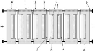
**Figure 1**. Schematic diagram of a bipolar plate stacked microbial fuel cell. Five single cells are connected in series. Anodic compartment contains *P. vulgaris*, glucose and thionin. Ferricyanide reduction is used as a cathodic reaction. 1. Bipolar plate made of graphite, 2. anode, 3. cathode, 4. RVC electrodes, 5. Nafion membrane, 6. anolyte, 7. catholyte, 8. end plates, 9. screws. Volume of each compartment is 26 mL.
