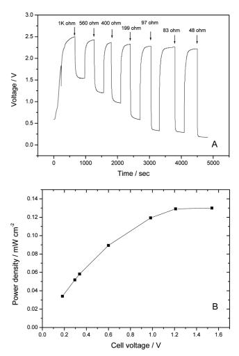
**Figure 4**. Voltage output as a function of different external loads for the five single cells stacked in series (panel A) and corresponding plot of power density *vs* cell voltage (panel B). Ferricyanide reduction reaction was utilized at a cathode. Volumes of anodic and cathodic compartments are 26 mL. Each anodic compartment contains 2 mL of *P. vulgaris* suspended solution, 6 mL of 1 mM thionin, 2 mL of 1 mM glucose, and 16 mL of buffer solution.
