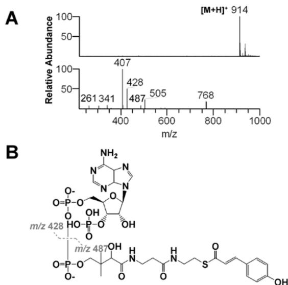
**Figure 2.** Mass spectrum and MS/MS fragment analysis of the *p*-coumaric acid reaction product with R4CL2. A, Mass and MS/MS spectrum of the *p*-coumaric acid reaction product; B, identified fragments of *p*-coumaroyl CoA by MS/MS analysis.
