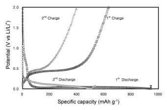
**Figure 4.** Potential as a function of specific capacity for Fe(1)Cu (1)Si(3.5)/Graphite composite.
