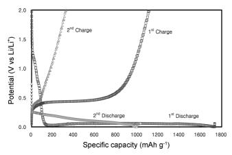
**Figure 3**. Potential as a function of specific capacity for Fe(1)Cu (1)Si(3.5) composite.
