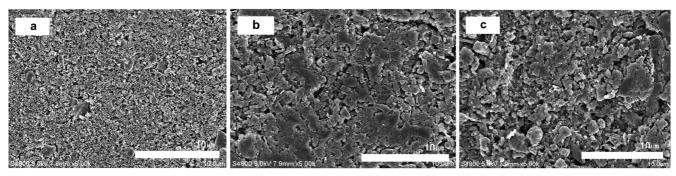
Figure 2. SEM pictures for the electrodes with compositions, a) Fe (1)Cu(1)Si(3.5) composite with SPB, b) Fe(1)Cu(1)Si(3.5)/Graphite composite, c) Fe(1)Cu(1)Si(2.5)/Graphite composite.
