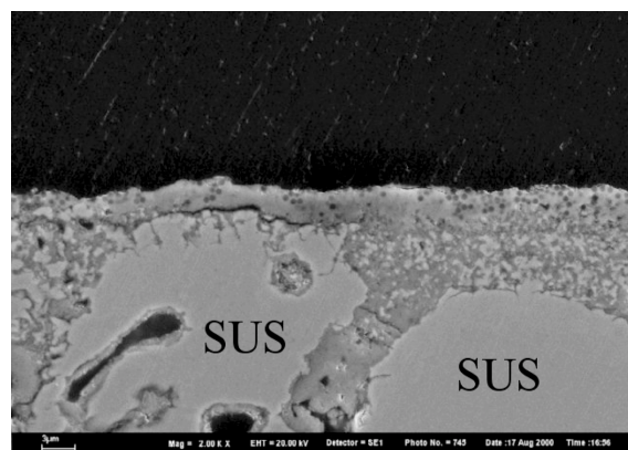
Figure 4. SEM image of cross-section of the SiO 2 (150 nm)/SiO 2 (500 nm)/Ni-SUS support.
