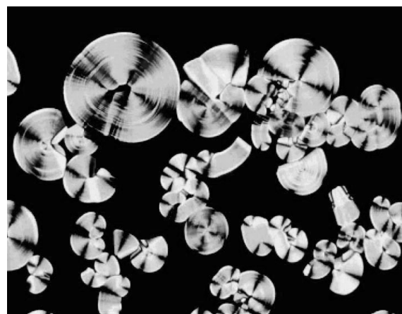
Figure 11. Optical polarized micrograph (100x) of the texture by the 3-D honeycomb-like lamellar liquid crystalline phase of 17 at 149 °C on the cooling scan.
