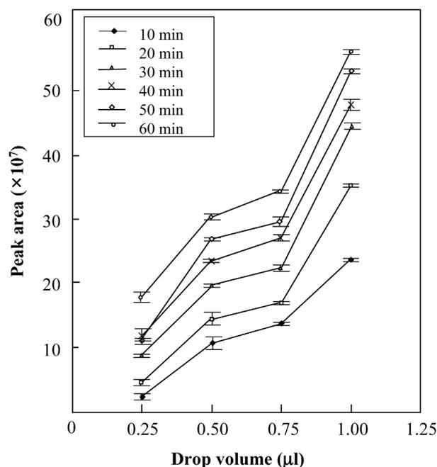
**Figure 3.** Effect of drop volume and extraction time on the analytical signal in HS-HD-LPME.
