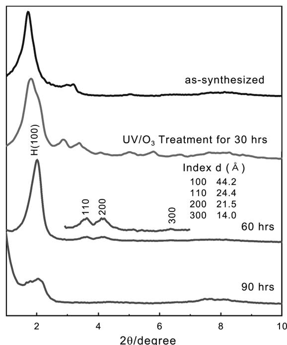
**Figure 6.** Powder XRD pattern of the samples obtained by UV/O<sub>3</sub> treatment of hexagonal  $P6m$  structure at various times.
