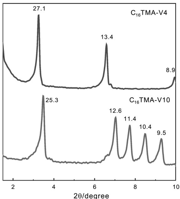
Figure 1. Powder XRD pattern of  $C_{16}$ TMA-Vanadate composite.
