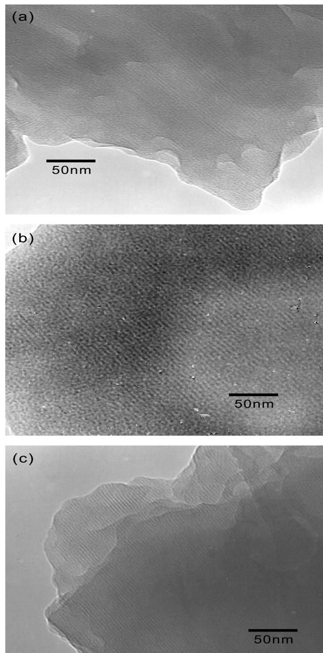
**Figure 5.** Transmission electron microscope image of (a) hexagonal  $P6m$  structure, obtained from C16TMA-V4, (b) cubic  $Fm3m$  structure from C16TMA-V4 and (c) cubic  $Fd3m$  structure from C16TMA-V10.
