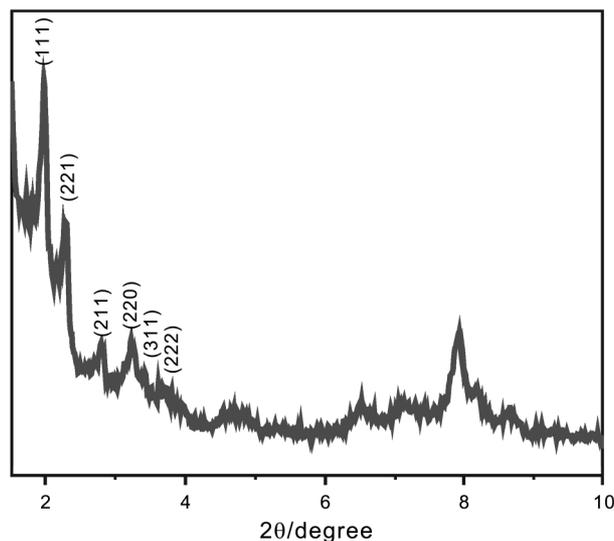
Figure 4. Powder XRD pattern of cubic mesostructured vanadium oxide, obtained from  $C_{16}$ TMA-V10.
