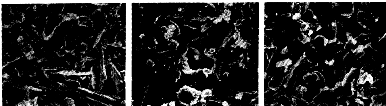
Figure 6. SEM photographs of the \text{Bi}_{2-x}\text{Mo}_x\text{Sr}_2\text{Ca}_2\text{Cu}_3\text{O}_y system with x = 0.07 , 0.10 and 0.30 , respectively.
