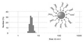
**Figure 1**. Hydrodynamic size distribution of <sup>MAA</sup>QD in aqueous solution prepared and used in this study.
