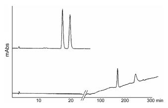
**Figure 1**. Chromatograms of enantiomer separation of *N*-FMOC valine on Chiralcel OJ-H (the top) and Chiralcel OD-H (the bottom) under reversed phase conditions. The chromatographic conditions are given in Tables 1 and 2.
