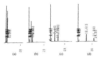
**Figure 2**. Separation of 2,2,2-trifluoro-1-(9-anthryl)ethanol (S2) enantiomers on CSP 1. Flow rate; 1.2 mL/min. Mobile phase (a) 20% isopropylalcohol (IPA) in heptane (b) 10% IPA in heptane (c) 5% IPA in heptane (d) 2.5% IPA in heptane.
