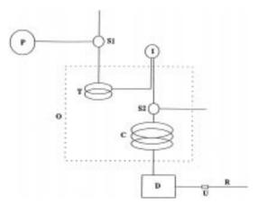
**Figure 1.** Schematic diagram of open tubular capillary column ion chromatographic system: **P**, IC pump; **S1**, first splitter; **S2**, second splitter; **I**, injector; **T**, preheating tube; **C**, column; **D**, detector; **R**, restrictor; **O**, GC oven; **U**, union.
