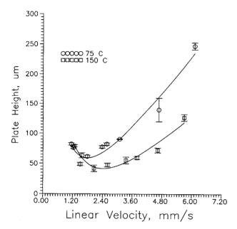
**Figure 2.** Van Deemter curves at 75  $^{\circ}$ C and 150  $^{\circ}$ C. (column: 1m×50  $\mu$ m i.d. capillary coated with Latex particles, eluent: 1mM sodium sulfate, detector: UV detector at 210 nm).
