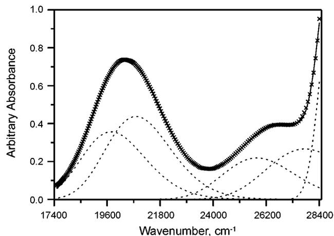
**Figure 1.** Resolved electronic absorption spectrum of *cis*-[Cr(cyclam)(NCS)<sub>2</sub>]<sup>+</sup> in aqueous solution at 298 K.
