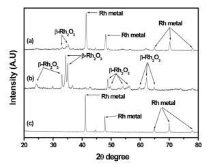
Figure 1. XRD patterns of rhodium black, as received (a); oxidation in air at 800 °C for 5 h (b); reduction under  $96\%-N_2/4\%-H_2$  mixture gas at 900 °C for 5 h (c).
