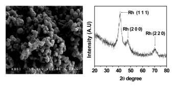
**Figure 3**. SEM image of the compound recovered by cementation (left) and its XRD pattern (right).
