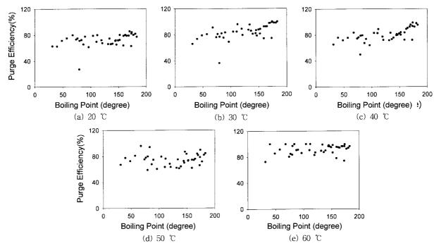
Figure 5. Purge efficiencies of VOCs according to boiling points of each compound at sample temperature (20, 30, 40, 50, 60 °C).
