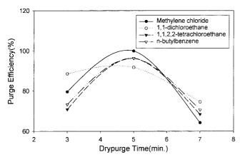
**Figure 6**. Purge efficiencies of VOCs according to change of dry purge times at purge time/sample temperature. (11 min/60 °C).
