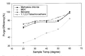
**Figure 4**. Purge efficiencies of VOCs according to change of sample temperature at purge time/drypurge time (11 min/5 min).
