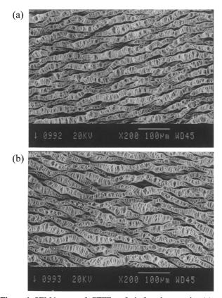
**Figure 1**. SEM images of ePTFE grafts before drug coating (a) and after drug coating (b).
