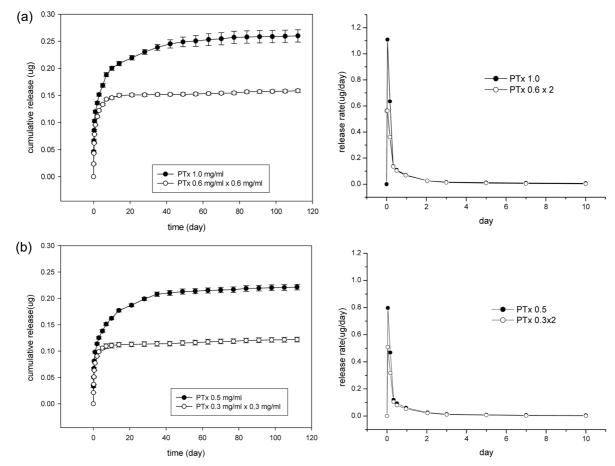
**Figure 3**. Drug release kinetics. Each curve represents 5 grafts (p < 0.05). (a) Cumulative release and release rate of a single dipping (in 1.0 mg/mL) and double dipping (in 0.6 mg/mL  $\times$  2) with a total loading amount of about 0.75  $\mu$ g/mm<sup>2</sup>. (b) single (0.5 mg/mL) vs double (0.3  $\times$  2 mg/mL) with about 0.4  $\mu$ g/mm<sup>2</sup>.
