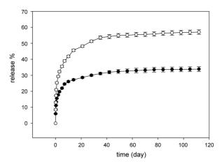
**Figure 2**. In vitro release % profile of PTx from a eFTFE graft containing 0.75  $\mu$ g/mm<sup>2</sup> (open circle) and 0.38  $\mu$ g/mm<sup>2</sup> (closed circle) after single dippining. Data are an average of grafts (p < 0.05, statistically significant).
