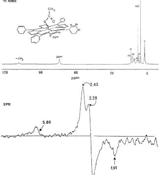
**Figure 2.** <sup>1</sup>H NMR (360 MHz) and EPR spectra for the reaction of  $(d_8$ -TPP)Fe(III)O\_3SCF<sub>3</sub> with 1.0 equiv. [CH<sub>3</sub>C(=O)S]<sup>-</sup>K<sup>+</sup>/methanol in dichloromethane solution. EPR spectrum was recorded at 77 K with 6000 G sweep, 9.19 GHz, 100 KHz modulation at 5 mwatt.
