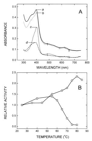
**Figure 2**. (A) Absorption spectra of HRP encapsulated in silica glass (a, b) and in aqueous solution (c, d) at 25 °C (a, c) and 80 °C (b, d). The HRP concentration was 5  $\mu$ M in 100 mM phosphate buffer (pH 7). Other conditions were the same as those in Figure 1A. (B) Catalytic activities of HRP in solution (*squares*) and encapsulated HRP (*circles*) as a function of temperature. The activity at 25 °C was set to 1.
