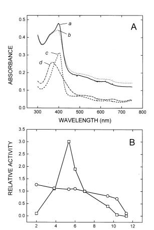
**Figure 1**. (A) Absorption spectra of HRP encapsulated in silica glass (a, b) and in aqueous solution (c, d) at pH 7 (a, c) and pH 2 (b, d). The spectra were obtained in a cuvette with 1 cm pathlength using a diode array spectrophotometer. The HRP concentration was 5  $\mu$ M in 100 mM phosphate buffer. (B) Catalytic activities of HRP in solution (*squares*) and encapsulated HRP (*circles*) as a function of pH. The activity at pH 7 was set to 1.
