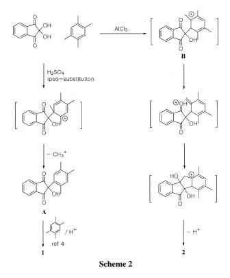
intermediate **B** was formed. **B** was transformed into the tetracyclic indenoindanone derivative **2** as shown in Scheme 2 and in our previous report<sup>4</sup> in the reaction conditions.
