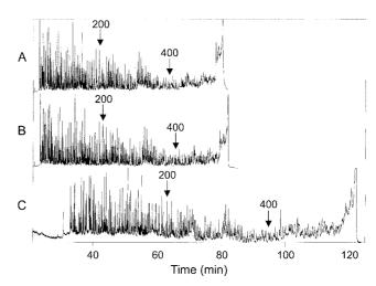
**Figure 2**. The electropherograms at various concentrations of PEO gel matrix. (A) 1.8% of Mr 8,000,000 and 1.4% of Mr 600,000, (B) 2.0% of Mr 8,000,000 and 1.4% of Mr 600,000, (C) 2.3% of Mr 8,000,000 and 1.5% of Mr 600,000. The electric field employed was 200 V/cm, but other conditions were the same as shown in Figure 1.
