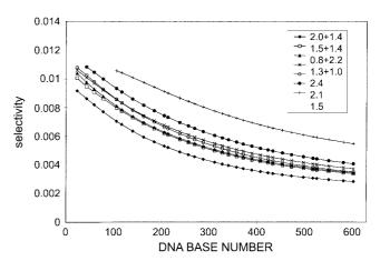
**Figure 3**. The mobility of single-stranded DNAs at different combinations of PEO gel matrices. The composition of gel matrix is shown in the small box and y-axis represents the mobility (cm<sup>2</sup>/Vsec). The larger the mobility difference is, the better the separation efficiency is. The electric field employed was 150 V/cm and other conditions were the same as shown in Figure 1.
