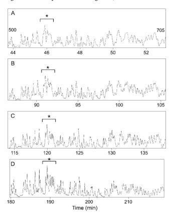
**Figure 4**. The electropherograms of PGEM/U standard sample. Only DNA bases between 500 base and 705 base region is shown for comparison. An effective capillary length of (A) 25 cm, (B) 50 cm, (C) 79 cm, (D) 100 cm. The G, C rich region is marked by \*in order to clarify the improvement of resolution as the effective length of the capillary increased.
