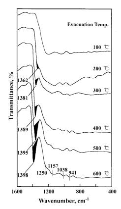
Figure 1. Infrared spectra of  $NiSO_4/\gamma$ -Al<sub>2</sub>O<sub>3</sub> evacuated at different temperatures.
