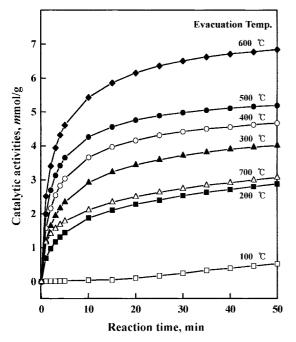
Figure 2. Catalytic activities of  $NiSO_4/\gamma Al_2O_3$  for ethylene dimerization as a function of evacuation temperature.
