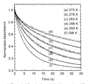
**Figure 1**. Theoretical fit to the thermal bleaching reaction of PMC form of SNO doped in PS. For all different temperatures, same fitting parameters were used. The dotted lines are experimental data and the solid lines represent fits obtained using Eq. (1). The fitting parameters are listed in Table 1.
