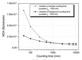
**Figure 8**. MDA values of <sup>239,240</sup>Pu, <sup>238</sup>Pu plotted *vs* variation of the sample and the background counting time.
