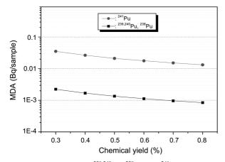
**Figure 7**. MDA values of <sup>239,240</sup>Pu, <sup>238</sup>Pu and <sup>241</sup>Pu plotted *vs* the chemical yield.
