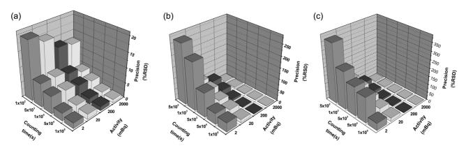
Figure 2. Variation of precision (% RSD) observed for alpha spectrometry (a), alpha/beta gross counting (b) and liquid scintillation counting (c).
