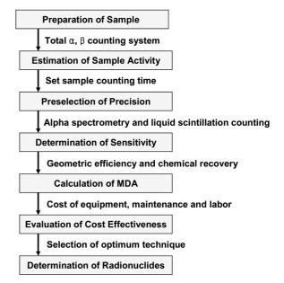
Figure 1. Parameters affecting the sensitivity of the determination of the Pu isotopes.
