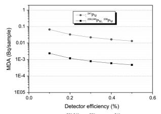
**Figure 6.** MDA values of <sup>239,240</sup>Pu, <sup>238</sup>Pu and <sup>241</sup>Pu plotted *vs* the detector efficiency.
