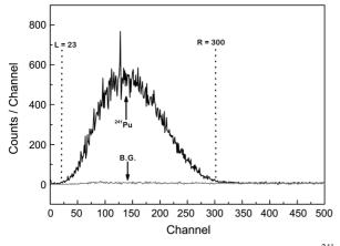
**Figure 3.** Left and Right channel in the beta spectrum of <sup>241</sup>Pu standard source [16].
