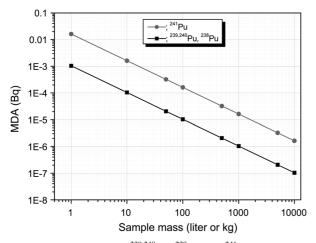
**Figure 4**. MDA values of  $^{239,240}$ Pu,  $^{238}$ Pu and  $^{241}$ Pu plotted *vs* the sample mass.
