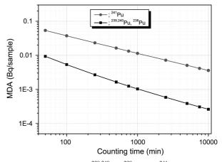
**Figure 5**. MDA values of  $^{239,240}$ Pu,  $^{238}$ Pu and  $^{241}$ Pu plotted *vs* the counting time.
