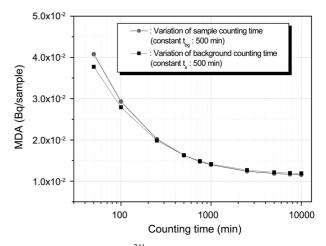
**Figure 9.** MDA values of  $^{241}$ Pu plotted *vs* variation of the sample and the background counting time.
