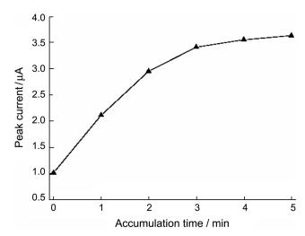
**Figure 5**. Influence of accumulation time on the oxidation peak current of  $5.0 \times 10^{-7}$  mol/L 6-BAP. Other conditions are the same as in Fig. 3c.
