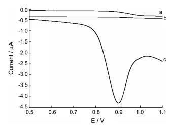
**Figure 3**. DP voltammograms of  $5.0 \times 10^{-7}$  mol/L 6-BAP in 0.1 mol/L phosphate buffer (pH 7.0) after 3-min open-circuit accumulation. (a): at unmodified GCE, (b): at DCP film modified GCE, and (c): at SWNT-DCP modified GCE. The DPV parameters: pulse amplitude = 50 mV, scan rate = 20 mV/s, pulse width = 50 ms.
