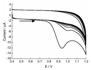
**Figure 2**. Successive cyclic voltammograms of  $5.0 \times 10^{-6}$  mol/L 6-BAP at SWNT-DCP modified GCE in 0.1 mol/L phosphate buffer (pH 7.0). Scan rate: 100 mV/s.
