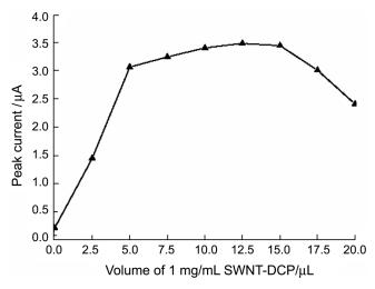
**Figure 4**. Effect of the volume of the SWNT-DCP suspension on the oxidation peak current of  $5.0 \times 10^{-7}$  mol/L 6-BAP. Other conditions are the same as in Fig. 3c.
