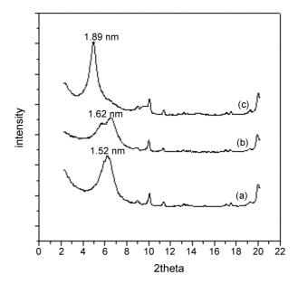
**Figure 2.** XRD patterns of HMMT treated with APS-ethanol solution. (a) 0.01APS-MMT, (b) 0.05APS-MMT and (c) 0.1APS-MMT
