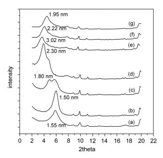
**Figure 4.** XRD patterns of HMMT treated simultaneously with APS and DDA in ethanol. (a) 0.01DDA-0.01APS-MMT, (b) 0.05DDA-0.05APS-MMT, (c) 0.1DDA-0.1APS-MMT, (d) 0.3DDA-0.01APS-MMT (e) 0.5DDA-0.01APS-MMT (f) 0.5DDA-0.05APS-MMT, and (g) 0.5DDA-0.1APS-MMT.
