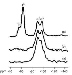
**Figure 6**. <sup>29</sup>Si CP MAS NMR spectra of (a) HMMT, (b) 0.1APS-MMT and (c) 0.3DDA-0.01APS-MMT.
