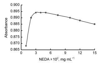
**Figure 3.** Effect of NEDA concentration on the absorbance: potassium iodate, 3  $\mu$ g mL<sup>-1</sup>; hydrochloric acid, 0.025 mol L<sup>-1</sup>; hydroxylamine, 0.25 mg mL<sup>-1</sup>; Sulfanilic acid, 0.2 mg mL<sup>-1</sup>.
