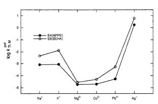
**Figure 4.** Effect of plastisizer on selectivity coefficients,  $\log k^{\text{pot}}_{TL,M}$  for the Tl<sup>+</sup>-ISEs (E4 & E6 in Table 1) based on L<sub>3</sub>.
