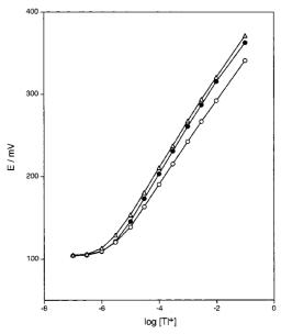
**Figure 2.** Potential responses of calix[4]pyrroles-based Tl<sup>+</sup>-ISEs:  $(\triangle)$  E1,  $(\bigcirc)$  E2 and  $(\bullet)$  E4 in Table 1, respectively.
