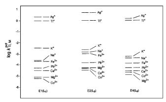
**Figure 3**. Selectivity coefficients, log  $k^{\text{pot}}_{\text{TI,M}}$  for the TI<sup>+</sup>-ISEs based on L<sub>1</sub>-L<sub>3</sub> with NPPE as plasticizer.
