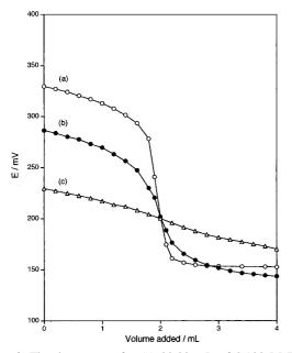
Figure 6. Titration curves for (a) 20.00 mL of 0.100 M TINO<sub>3</sub> with 1.00 M KI; (b) 20.00 mL of 0.010 M TINO<sub>3</sub> with 0.10 M KI; (c) 20.00 mL of 0.0010 M TINO<sub>3</sub> with 0.010 M KI by using the TI<sup>+</sup>-ISE (E4 in Table 1).
