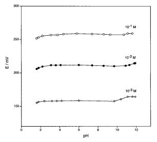
**Figure 5.** Effect of pH on the EMF response of the  $Tl^+$ -ISE (E4 in Table 1). HNO<sub>3</sub> and KOH were used to change the pH.
