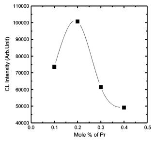
**Figure 3**. Maximal peak CL intensity at 614 nm of CaTiO<sub>3</sub>:Pr, Ga (1 mole %) with various Pr mole%. (anode voltage and current: 1 kV, 20  $\mu$ A)
