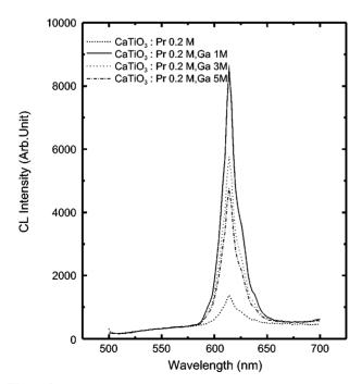
**Figure 2.** CL intensity of Ga(*x*)-doped CaTiO<sub>3</sub>:Pr (x = 1, 2, 3 mole %). (anode voltage and current: 1 kV, 20  $\mu$ A)
