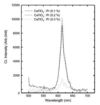
**Figure 1**. CL intensity of CaTiO<sub>3</sub>:Pr with various Pr mole%. (anode voltage and current: 1 kV,  $20 \mu \text{A}$ )
