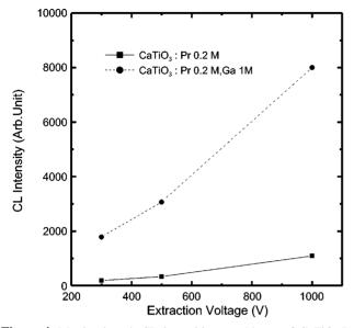
**Figure 4.** Maximal peak CL intensities at 614 nm of CaTiO<sub>3</sub>:Pr (0.2%), Ga (1%) and CaTiO<sub>3</sub>:Pr (0.2%) with various anode voltages. (anode current:  $20 \ \mu$ A)
