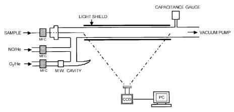
Figure 1. Experimental set-up of the discharge flow-chemiluminescence imaging system.
