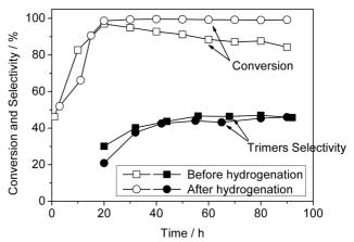
**Figure 3.** Effect of hydrogenation of NCC feed on the isobutene conversion and trimers selectivity. The WHSV and temperature were  $5 \, h^{-1}$  and  $70 \, ^{\circ}$ C, respectively.
