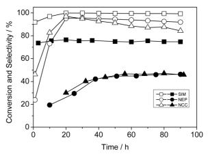
Figure 1. The isobutene conversion (empty symbols) and trimers selectivity (filled symbols) depending on the feed and time-onstream. The WHSV values for SIM, NEP and NCC are 10, 5 and 5 h<sup>-1</sup>, respectively.
