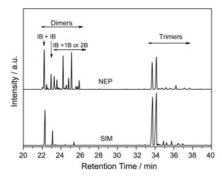
**Figure 2.** Gas chromatograms in the regions for dimers and trimers (time-on-stream: 100 h) obtained by the oligomerization of SIM and NEP feeds. IB, 1B and 2B represent isobutene, 1-butene and 2-butene, respectively.
