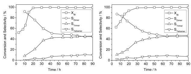
**Figure 4.** The isobutene conversion and selectivities for dimers, trimers and tetramers after the hydrogenation of NCC feed (left) and NEP feed (right). The WHSV and temperature were 5  $h^{-1}$  and 70 °C, respectively.
