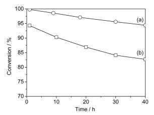
**Figure 5**. Effect of hydrogenation of the NEP feed on the recovery of the activity and deactivation rate after activation: (a) with hydrogenation; (b) without hydrogenation. The WHSV and temperature were 5  $h^{-1}$  and 70 °C, respectively.
