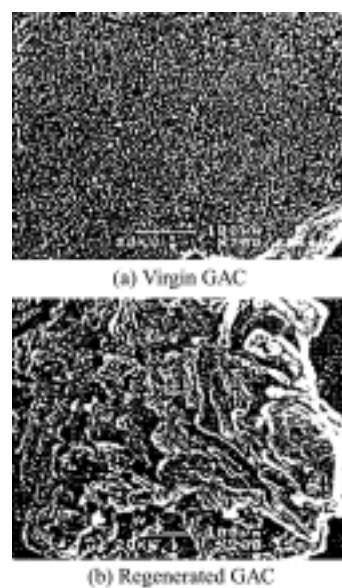
Figure 6. Scanning Electron Micrographs (SEMs) of (a) Virgin and (b) Regenerated GAC (200 X Magnification).
