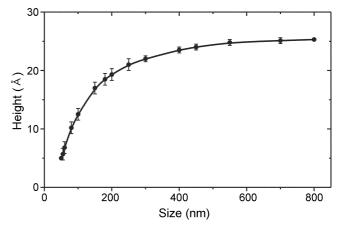
**Figure 3.** Island height as a function of island size for the 400 different SAMs-coated samples prepared from the OTS solutions of various concentrations (0.1-10 mM) and for various amounts of SAMs growth time (1-100 s).
