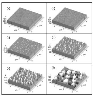
**Figure 1.** TM-AFM images of the time-resolved sequence of partial SAMs growth at  $10 \,^{\circ}$ C. (a) 1 s, (b) 3 s, (c) 7 s, (d) 12 s, (e) 30 s, (f) 100 s.
