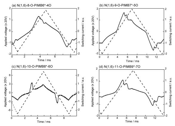
**Figure 3**. The polarization reversal current in the B2 phase: (a) N(1,6)-8-O-PIMB6\*-4O at 130 °C under the application of 66  $V_{PP}$  triangular wave of 13.5 Hz, (b) N(1,6)-9-O-PIMB7\*-5O at 140 °C under the application of 80  $V_{PP}$  triangular wave of 8.2 Hz, (c) N(1,6)-10-O-PIMB8\*-6O at 140 °C under the application of 260  $V_{PP}$  triangular wave of 12.8 Hz, (d) N(1,6)-11-O-PIMB9\*-7O at 130 °C under the application of 72  $V_{PP}$  triangular wave of 8.7 Hz.
