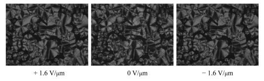
**Figure 6**. Photomicrographs showing the switching behavior in the B2 phase in a 6.2  $\mu$ m thick cell of N(1,6)-10-O-PIMB8\*-6O at 130 °C. SmC<sub>A</sub>P<sub>F</sub>\* ( $E = 0 \text{ V } \mu\text{m}^{-1}$ ) switches to SmC<sub>A</sub>P<sub>F</sub>\* under  $E = \pm 1.6 \text{ V } \mu\text{m}^{-1}$  under the application of an electric field with a slight change of birefringence color.
