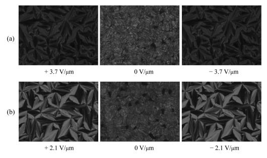
**Figure 5**. Photomicrographs of the switching behavior in the B2 phase: (a) 5.3  $\mu$ m thick cell of N(1,6)-9-O-PIMB7\*-5O at 140 °C, (b) 9.4  $\mu$ m thick cell of N(1,6)-11-O-PIMB9\*-7O at 130 °C. Circular domains of SmC<sub>8</sub>P<sub>A</sub>\* (E=0 V  $\mu$ m<sup>-1</sup>) switch to SmC<sub>A</sub>P<sub>F</sub>\* under the application of an electric field.
