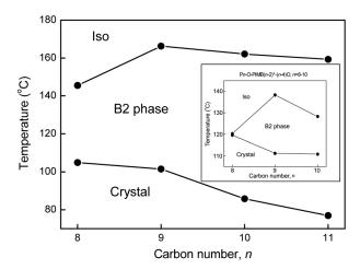
**Figure 1**. Phase diagram of the N(1,6)-n-O-PIMB(n-2)\*-(n-4)O series and Pn-O-PIMB(n-2)\*-(n-4)O series (in the inset) on cooling.
