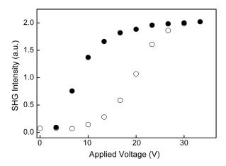
**Figure 4.** Electric field dependence of SHG intensity in a 5.3  $\mu$ m thick cell of N(1,6)-8-O-PIMB6\*-4O. A hysteresis curve was observed, indicating the field-induced antiferroelectric to ferroelectric phase transition. Open and closed circles stand for the data taken with increasing and decreasing voltage respectively.
