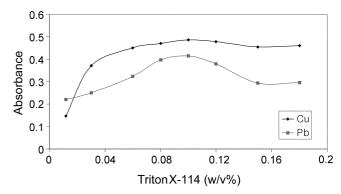
**Figure 2**. Effect of the Triton X-114 concentration on the CPE-preconcentration performance: Pb (50  $\mu$ gL<sup>-1</sup>) and Cu (20  $\mu$ gL<sup>-1</sup>); pH 5.8; Pyrogallol 1 × 10<sup>-4</sup> M.
