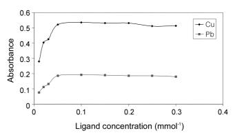
**Figure 3**. Effect of the Pyrogallol concentration on the CPE-preconcentration performance: Pb (50  $\mu$ gL<sup>-1</sup>) and Cu (20  $\mu$ gL<sup>-1</sup>); pH 5.8; Triton X-114 0.1% (w/v).
