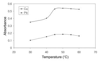
**Figure 4**. Effect of the temperature on the CPE-preconcentration performance: Pb (50  $\mu$ gL<sup>-1</sup>) and Cu(20  $\mu$ gL<sup>-1</sup>); pH 5.8; Triton X-114 0.1% (w/v); Pyrogallol 1 × 10<sup>-4</sup> mol dm<sup>-3</sup>.
