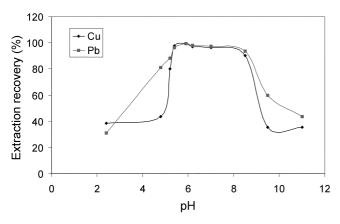
**Figure 1**. Effect of the pH on the CPE-preconcentration performance: Pb (50  $\mu$ gL<sup>-1</sup>) and Cu (20  $\mu$ gL<sup>-1</sup>); Triton X-114 0.1% (w/v); Pyrogallol 1 × 10<sup>-4</sup> M.
