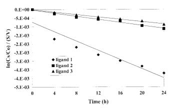
**Figure 1**. Kinetic plot of silver ion permeability as a function of time (h) through a PIM. Source phase: [AgNO<sub>3</sub>] = 10 mM; membrane phase [Ligands] = 10 mM; receiving phase: deionized water.
