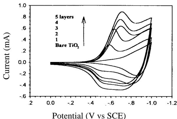
Figure 5. Cyclic voltammogram of BPPI layer on  $\text{TiO}_2$ .
