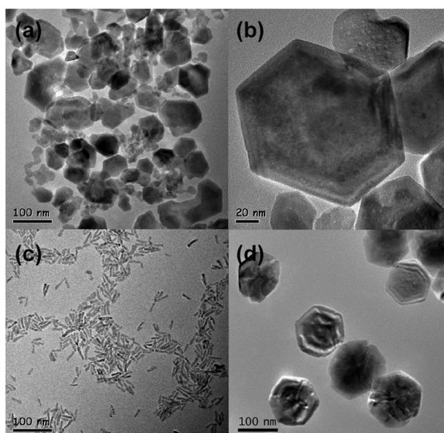
**Figure 3.** (a) The TEM image presents the hexagonal plate shapes of ZnO nanoparticles prepared by Method II. (b) The magnified TEM image (Method II) presents a clear view of the hexagonal shapes of ZnO nanoparticles. (c) The TEM image presents the nanorod shapes of ZnO nanoparticles prepared by Method III. (d) The TEM image presents the hexagonal cone shapes of ZnO nanoparticles prepared by Method I.
