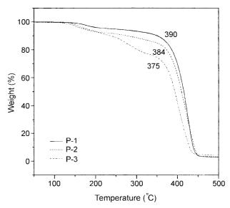
**Figure 3**. TGA thermograms of P-1, P-2, and P-3. The heating rate was 20 °C/min under a nitrogen atmosphere.
