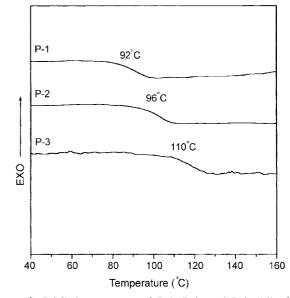
Figure 2. DSC thermograms of P-1, P-2, and P-3. All of the thermograms were obtained from the second heating scans and the scan rate was  $10 \text{ }^{\circ}\text{C/min}$ .
