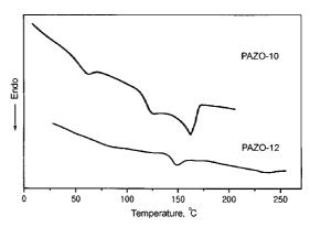
Figure 1. DSC thermograms of PAZO-10 and PAZO-12 (nitrogen atmosphere, heating rate: 10 °C/min.)
